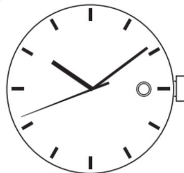
1. Pull the crown out two clicks then rotate the crown until the current time is displayed.
