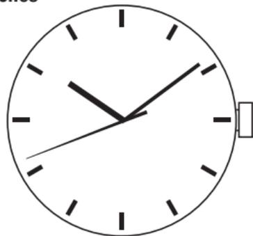
1. Pull the crown out one click then rotate the crown until the current time is displayed.
