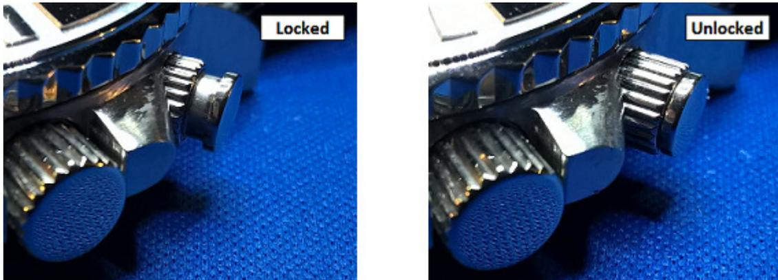
**To unlock:** unscrew the collar by rotating it counterclockwise until it is flush with the underside of the button.
